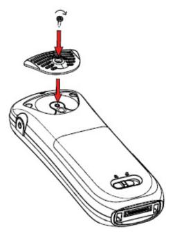
Figure 11: Screw the Cover into Position
