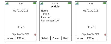
Figure 7: The system profile overrides the settings changed by the user
