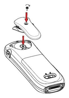
Figure 9: Screw the Hinge-type Clip into Position
