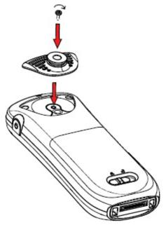
Figure 10: Screw the Swivel-type Clip into Position
