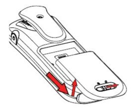
Figure 8: Easy Replaceable Battery - Unlock the Lid and Remove the Battery
